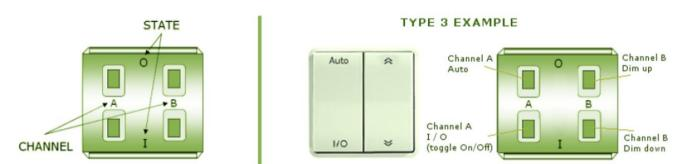
The button naming used below is referring to CHANNEL and STATE of the PTM200. Thus "Button AI" means STATE "I" on CHANNEL "A".
